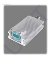
PLL LNB with AGC L.O. 9.75 is professional low noise block down converter with automatic gain control, wide dynamic range of up to 50 dB (biggest among any other LNB). AGC range of 25 dB, LO instability of 50 kHz, Gain (min) of 40 dB.
