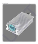
PLL LNB with AGC L.O. 11.25 is professional low noise block down converter with automatic gain control, wide dynamic range of up to 50 dB (biggest among any other LNB). AGC range of 25 dB, LO instability of 50 kHz, Gain (min) of 40 dB.
