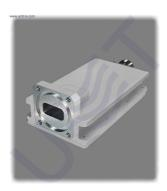
New PLL LNB with AGC is professional low noise block down converter with automatic gain control, wide dynamic range of up to 50 dB (biggest among any other LNB). AGC range of 25 dB, LO instability of 50 kHz, Gain (min) of 40 dB.
