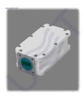
Ku-band LNB PLL with AGC LO 12.80 is low noise block down converter with automatic gain control. It is professional LNB with wide dynamic range - up to 50 dB (biggest among any other LNB). AGC range: 20 dB, LO instability: ±25 kHz, Gain (min): 34 dB.
