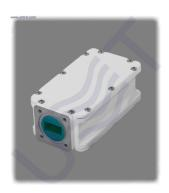
Ku-band LNB PLL with AGC LO 10.6 is low noise block down converter with automatic gain control. It is professional LNB with wide dynamic range - up to 50 dB (biggest among any other LNB). AGC range: 20 dB, LO instability:  $\pm 25 \text{ kHz}$ , Gain (min): 34 dB.
