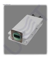
Ku-band LNB PLL dual LO 9.75 10.6 v.2 is Low Noise Block Down Converter with dual local oscillator 9.75 GHz and 10.6 GHz and dual 50 Ohm N-type output. LO instability: ± 2.5 ppm, Gain: 55 dB, Noise figure: 0.8 dB, Output power P1dB: 0 dBm.
