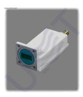
Ku-band LNB DRO LO 8.80 is Low Noise Block Down Converter with single LO 8.80 GHz and single 75 Ohm F-type output. LO instability: ± 2 MHz, Gain: 58 dB, Noise figure: 0.9 dB, Output power P1dB: +3 dBm.
