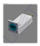
Ku-band LNB DRO LO 13.05 is Low Noise Block Down Converter with single LO 13.05 GHz and single 75 Ohm F-type output. LO instability: ± 2 MHz, Gain: 58 dB, Noise figure: 0.9 dB, Output power P1dB: +3 dBm.
