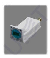
Ku-band LNB DRO LO 11.80 is Low Noise Block Down Converter with single LO 11.80 GHz and single 75 Ohm F-type output. LO instability: ± 2 MHz, Gain: 58 dB, Noise figure: 0.9 dB, Output power P1dB: +3 dBm.
