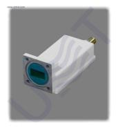
Ku-band LNB DRO LO 10.60 is Low Noise Block Down Converter with single LO 10.60 GHz and single 75 Ohm F-type output. LO instability:  $\pm$  2 MHz, Gain: 58 dB, Noise figure: 0.9 dB, Output power P1dB: +3 dBm.
