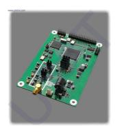
L-band DVB-S-S2-T modulator board is designed for DVB TS (transport stream) modulating, creating the L-band IF signal from parallel TS for further broadcasting in DVB-S, DVB-S2 or DVB-T standards.
