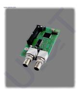
DVB ASI TS output board is designed to convert the parallel DVB TS into ASI TS and can be used with other our boards for building IP-ASI converters, receivers and other digital broadcasting equipment.
