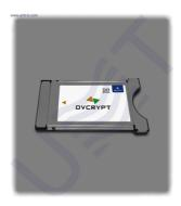
CAM is Conditional Access Module with common conditional access interface (Common Interface) in TVs and digital television receivers. The CAM allows to provide subscribers with access to encrypted content in digital television.
