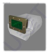
BUC-C04 is block up-converter with fixed output power P1dB 4 W (ALC power: 400 mW). BUC-C04 operates with up to 25 carriers and has built-in reference of 10MHz; ALC with 25 dB range; LEDs status indication at the rear side and integrated matched CWT.
