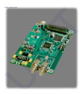
2 ch DVB-S-S2 receiver board is designed to convert the DVB-S/S2 IF (intermediate frequency in the L-band obtained from the LNB) to parallel DVB TS (transport stream).
